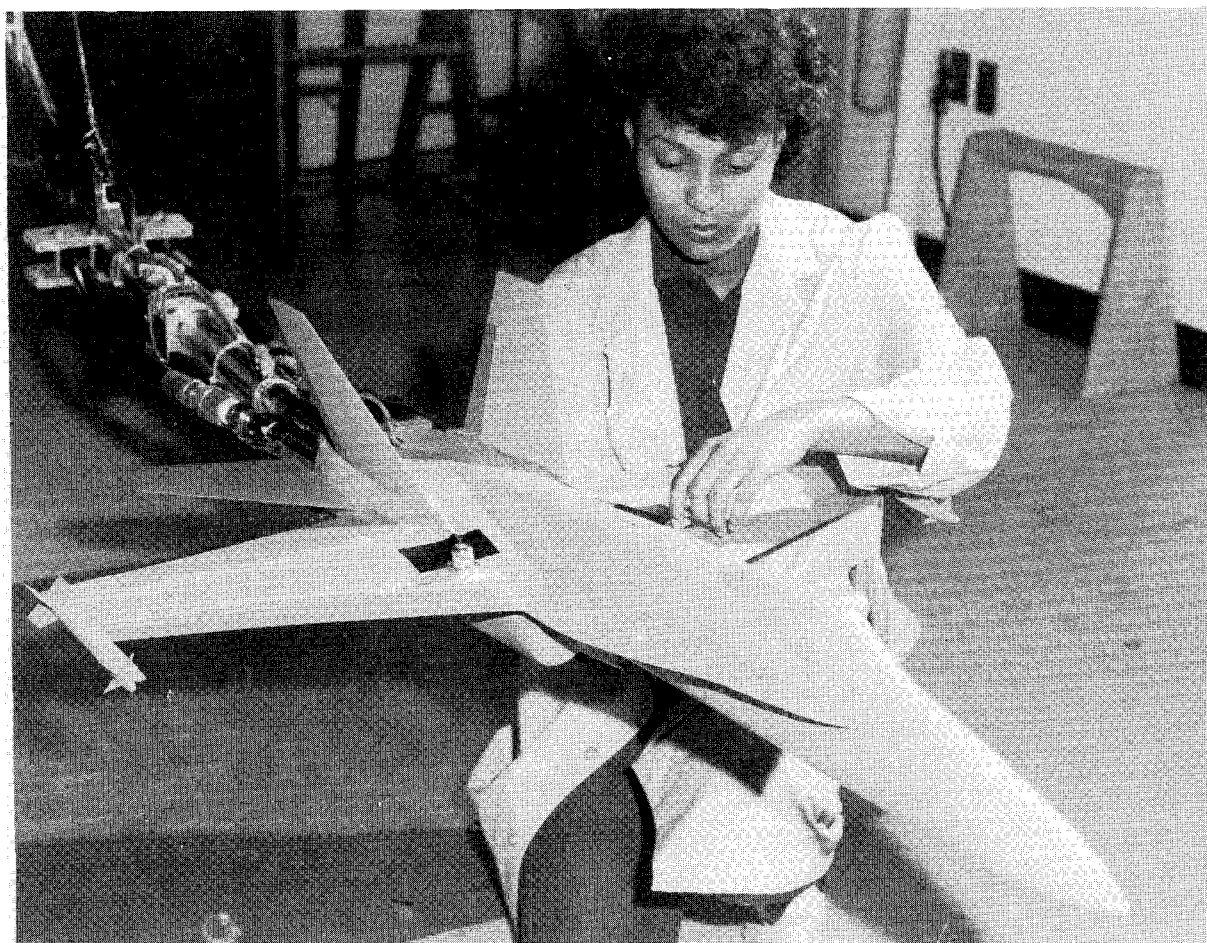
Fig. 4 F-18 model mounted in the VRF.
